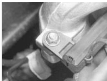
14.9b ... unbolt the wiring harness ...
