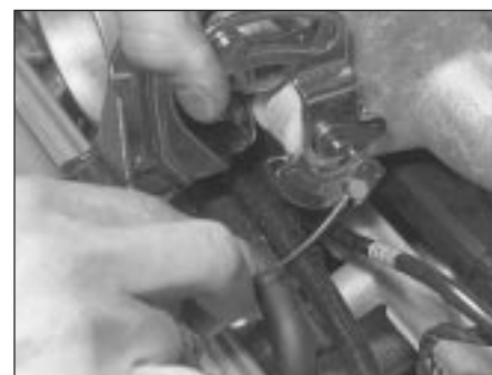
5.45 Accelerator cable retention arrangement at the throttle linkage
